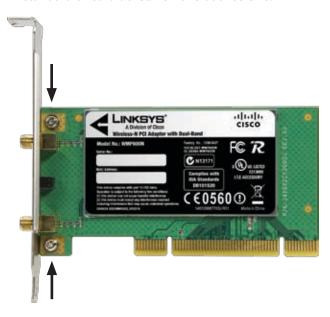
2. Use the two screws to attach the PCI board to the low-profile bracket.
